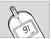
After 29 seconds, the Control Test result appears in the Display. Compare the result to the range listed on the end flap of your Test Strip carton. Using a tissue, remove the Test Strip and discard. The Meter will turn off automatically.
